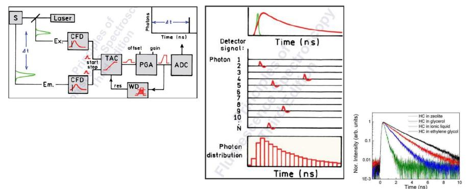
Fs time-resolved measurement - Broadband fluorescence up-conversion spectrograph
