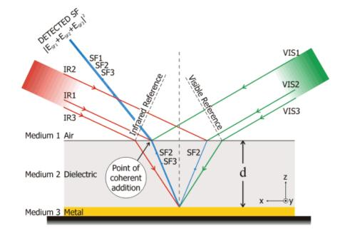
Schematic diagram of the composite dielectric/metal substrate. The three sum frequency beams generated in the point of coherent addition.
