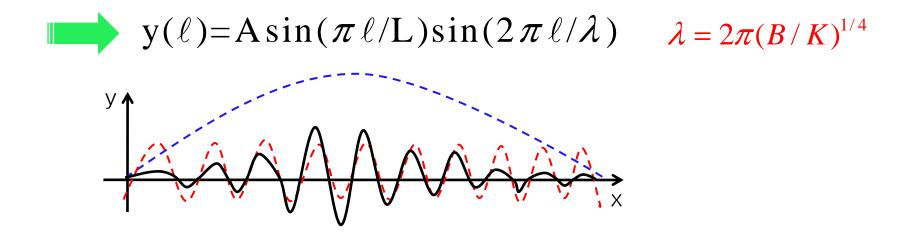
(1)  $\lambda = 2\pi (B/K)^{1/4}$ : The wavelength of the wrinkle when small amount of deformation occurs depend only on the property of film and substrate not the size of the system
