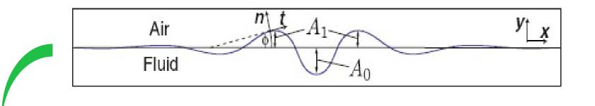
Total Energy: Bending energy of the film + gravitational energy of the subphase
