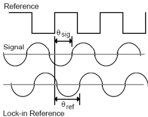
The SR850 amplifies the signal and then multiplies it by the lock-in reference using a phase-sensitive detector or multiplier. The output of the PSD is simply the product of two sine waves.
